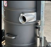
TAN Tangential inlet + cyclone
